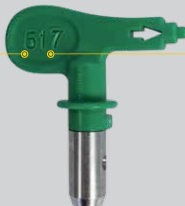
**Orifice diameter:** The orifice diameter (in this case, 0.017 inch) determines the flow volume and thus the amount of paint applied.
