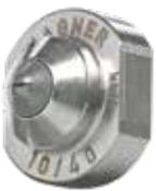
AirCoat pre-atomisation nozzles provide extra fine atomisation even with low inlet air pressure. This is especially important for processing water- or solvent-based paints. Using a pre-atomisation nozzle allows you to work with less material and air quantity. There is significantly less overspray and material consumption decreases. Compared to the standard AirCoat nozzle the material is pre-atomised directly at the outer edge of the nozzle. The result: an especially even and soft spray pattern.
