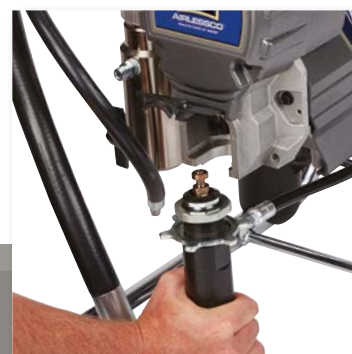
2. LIFT DOOR AND REMOVE PUMP
