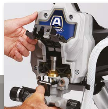
2. REMOVE PUMP SECTION
