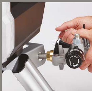
3. USE FRAME TO REMOVE CARTRIDGE
