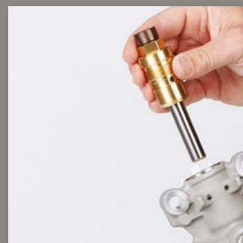
4. INSTALL NEW CARTRIDGE AND REPLACE PUMP
