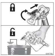
**NOTE:** If spray tip is difficult to rotate when turning to the unclog position, perform **Pressure Relief Procedure**, page 5, then turn Prime/Spray valve to spray position and repeat step 1.
