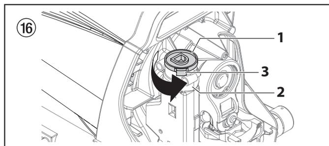
**i** If the stop (3) on the pressure switch prevents the knob bottom from continuing to turn, remove the knob bottom, re-orient it on the teeth and continue to turn it counterclockwise until it stops.
