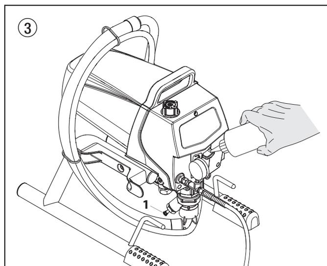
6. If equipped, fully depress the pusher stem (Fig. 3, item 1) to make sure the inlet ball is free.
