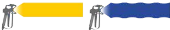
At low pressure: even spray jet from the diaphragm pump (yellow) and somewhat more irregular spray jet from the piston pump (blue).
